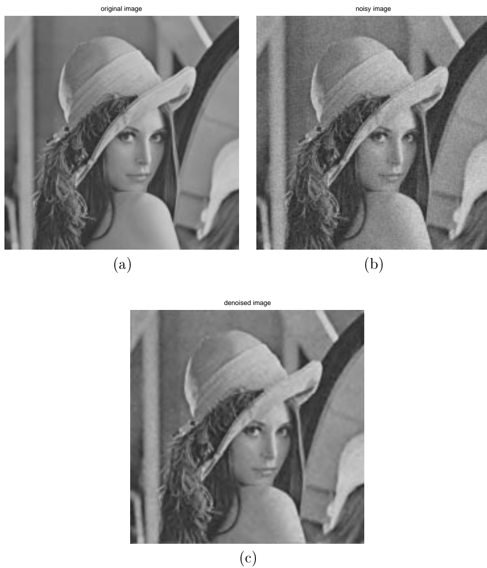
Figure 15: (a) Original Lena image ( 512 \times 512 \times 8bits ); (b) Noisy image (PSNR = 22.06 db). (c) Denoised Lena image using the proposed model (PSNR = 32.75 db).
